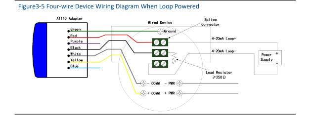
Figure 3-6 Four-wire Device Wiring Diagram When Loop Powered (with resistor)
